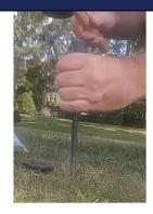
Using a Screw Driver, create a pilot hole
